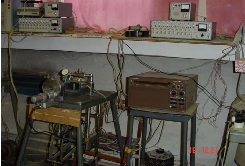
Figure 6 – Topaz-3-01 strain gage (1) and oscillograph H071.6M (2)
