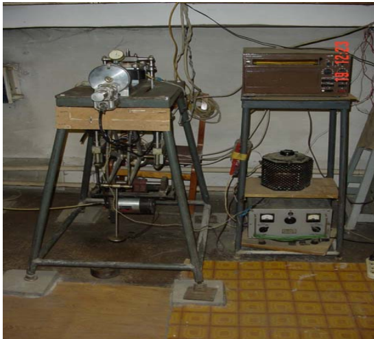
Figure 1 – Schematic diagram of the shifting device: 1 - holders of the shifting device; 2 - ground sample; 3 - loading frame; 4 - eccentric; 5 - the electric motor with a reducer; 6 - strain gauge of vertical load; 7 - strain gauge for moving the lower cage; 8 - strain gauge of horizontal force
