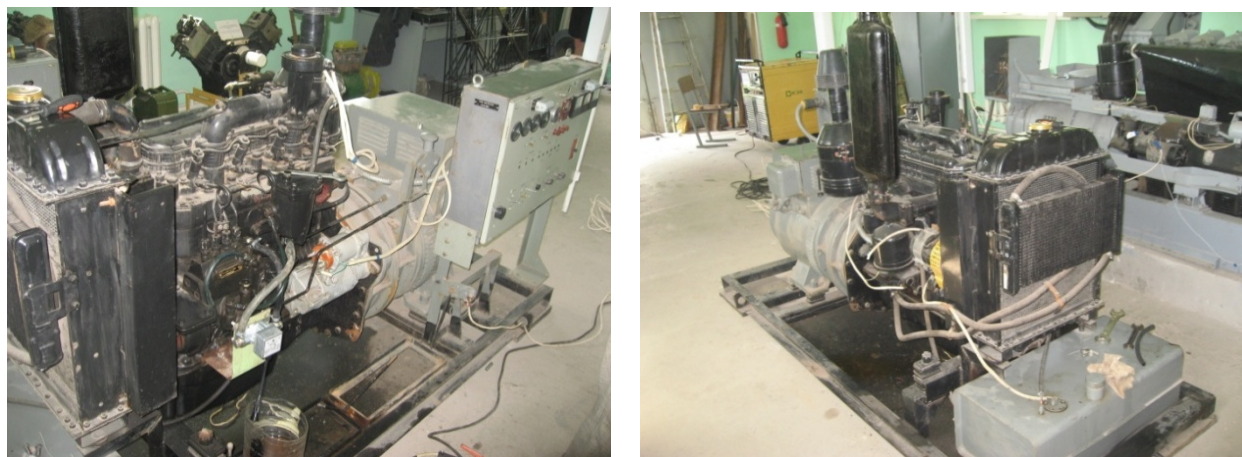
Figure 2 – Autonomic testing self-regulating lubrication system in diesel engine D-242
