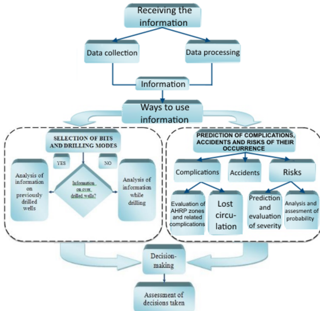
Figure 1 – Block diagram of obtaining and using information about drilling wells
