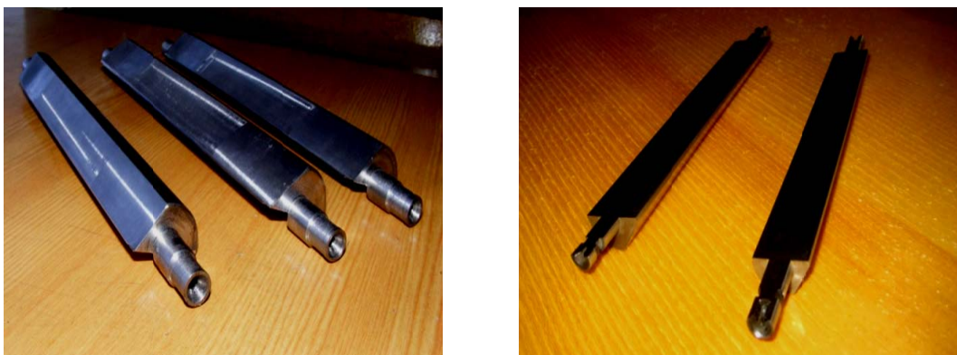
Figure 7 – Images of verification jigs
