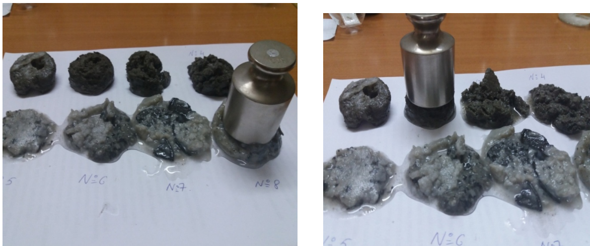
Figure 6 – Samples with the addition of micro-cement on a silicate base at various ratios of liquid glass and micro- cement
