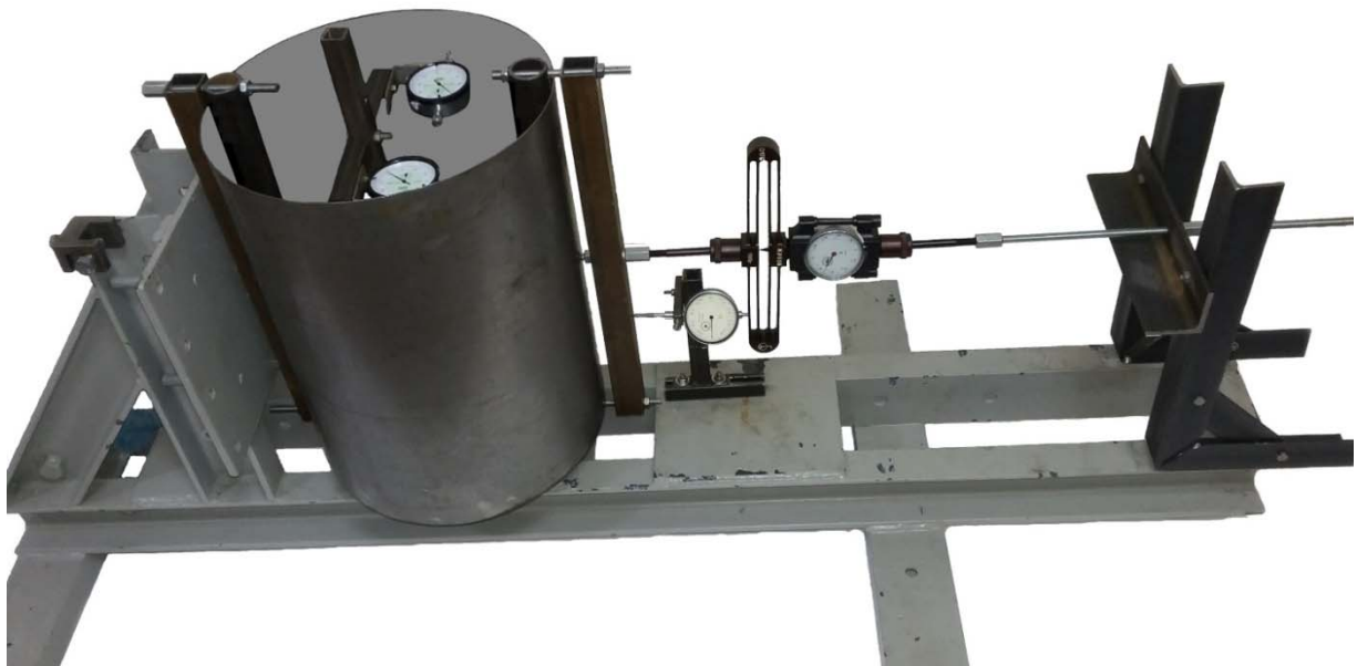
Figure 3 – Test stand for finding allowable displacement of flexible shell and its instruments
