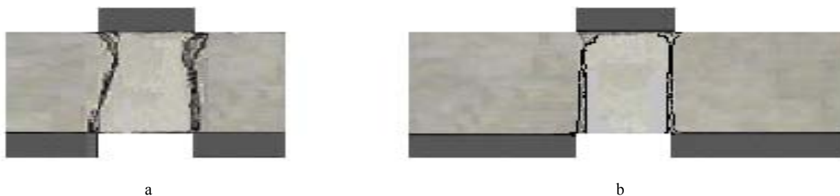
Figure 1 – Concrete beam fracture by shear (a) and tear (b)
