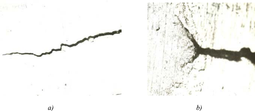
Figure 2 – The top of the fatigue crack: a) before the overload; b) after overload
