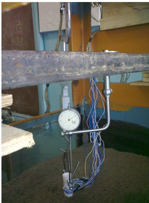
Figure 4 – General view of the model strain gauge static test pile pull out
