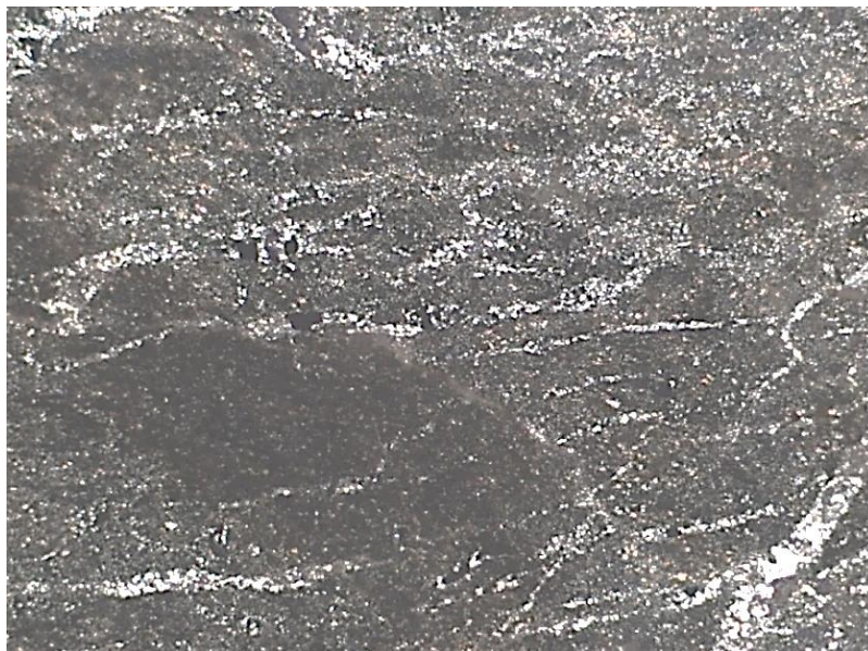
Figure 2 – Sericite-siliceous-carbanaceous shale, zoom 100 x , crossed nicols
