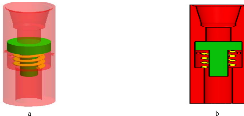
Figure 2 – Diagram of a hydroimpact apparatus. a - 3D, b - in section. Where: 1 – body; 2 - connecting adapter; 3 - valve; 4 - sanding rings; 5 - spring; 6 - nozzle holes.
