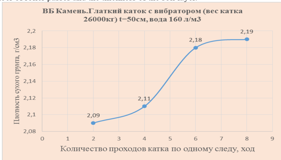
Figure 6 – Dependence graph of the dry soil density with a layer thickness of 50 cm on the passes number of a smooth roller (26000 kg.) with the vibrator turned on, water irrigation 160 l/m 3 , stone.
