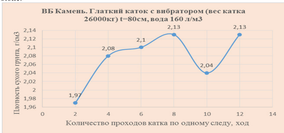
Figure 6 – Dependence graph of the dry soil density with a layer thickness of 50 cm on the passes number of a smooth roller (26000 kg.) with the vibrator turned on, water irrigation 160 l/m 3 , stone.
