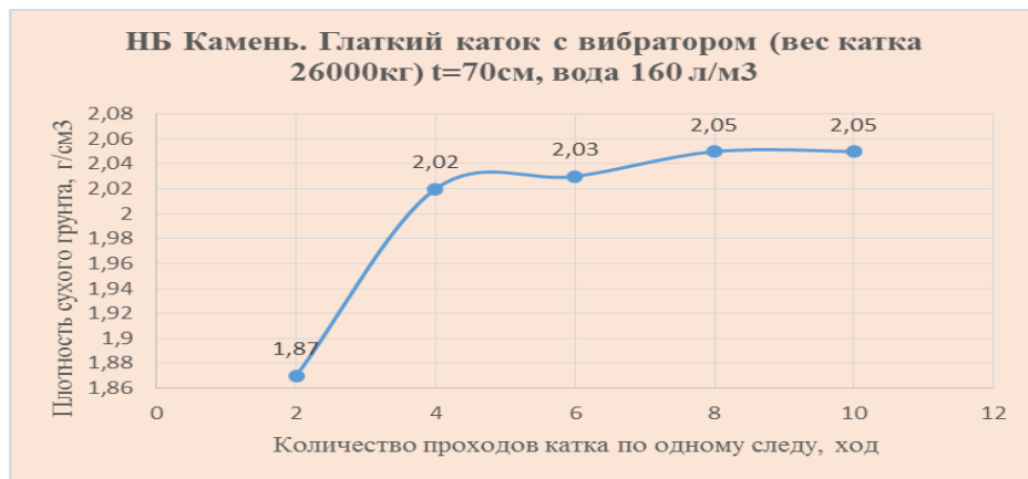
The number of passes of the rink on one track, stroke Figure 8 – Dependence graph of the dry soil density with a layer thickness of 70 cm on the passes number of a smooth roller (26000 kg.) with the vibrator turned on, water irrigation 160 l/m 3 , stone
