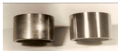
Fig. 3. Details before (on the left) and after (on the right) processing by the MAP method using LCTM SynHO-2M
