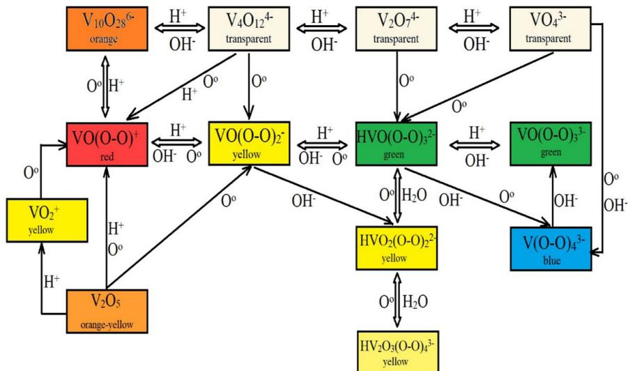
Fig. 1. Scheme of conversion of vanadium oxide compounds in solution
