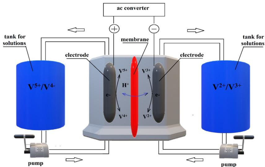
Fig.3. Structure of vanadium batteries
