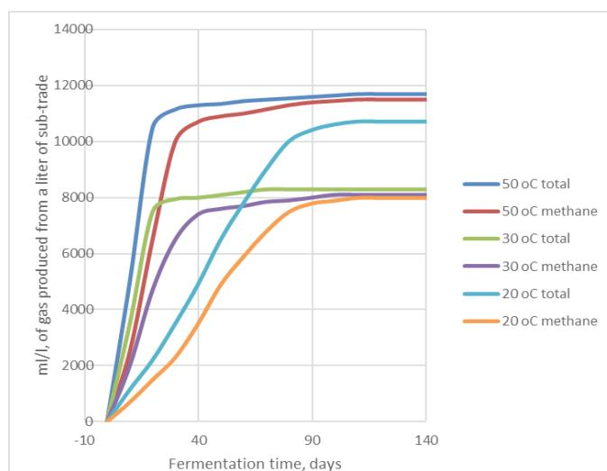
Fig. 2 – Effect of fermentation temperature and fermentation time on the amount of gas produced
