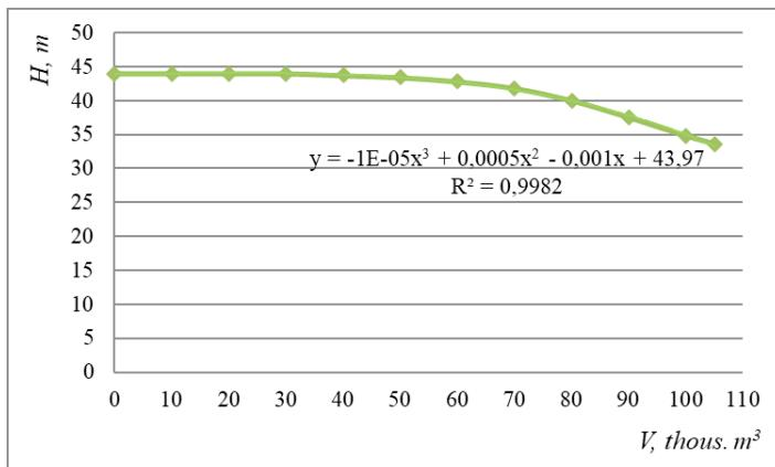
Fig. 4 - Dependence of the pump head value on the volume of abrasive material processed
