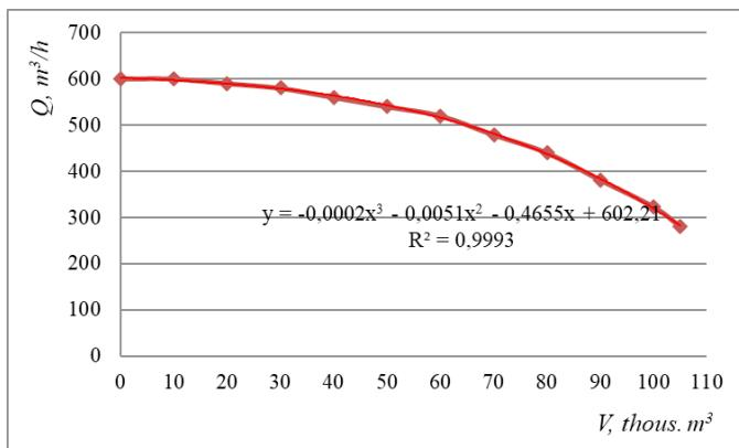
Fig. 3 - Pump flow rate as a function of the volume of abrasive material to be processed
