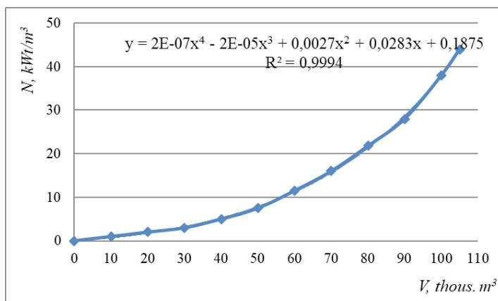
Fig. 2 - Energy consumption as a function of the volume of abrasive material to be processed
