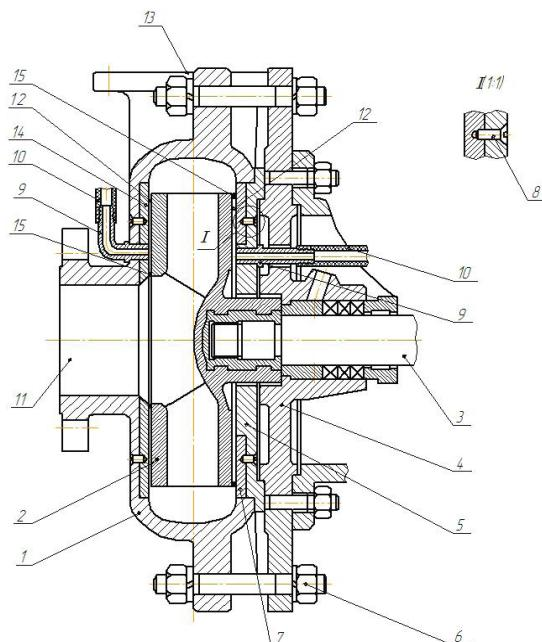
Fig. 7 - Working section of the soil pump with increased wear resistance:
