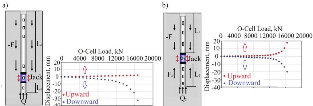
Fig. 3. Diagram of the jack location in the body of the piles: a) O-Cell jack is placed at the bottom; b) O-Cell jack is placed at mid-depth
