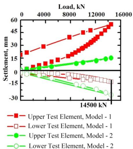
Fig. 8. The upward and downward load movement curves (model 1 and 2)
