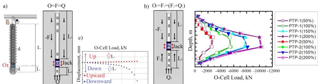
Fig. 2. Schematics of the O-cell method of pile load testing: a) typical gauge mechanisms and loads; b) typical load-transfer distributions (O-cell method); c) typical load-displacement (O-cell method)
