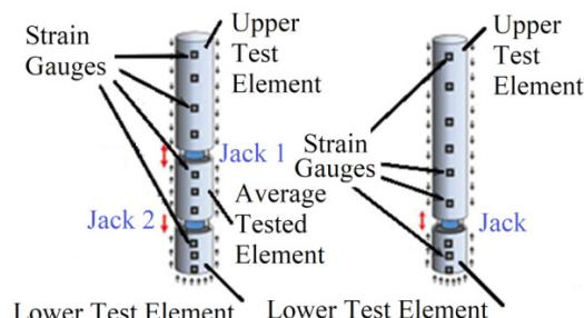
Fig. 1. Testing one level of jacks on the right and two levels of jacks on the left
