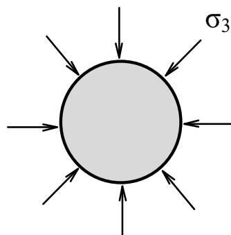
Fig. 4. Distribution of lateral ground pressure on the pile (Pile of circular cross section  $\sigma_3 = \text{const}$ )
