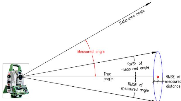
Fig. 1 - Determination of measurement error with electronic total station
