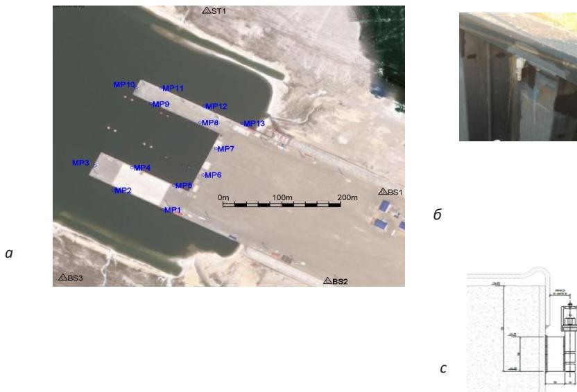
Fig. 3: a- Scheme of installation of monitoring points on berths;
