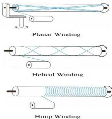
Figure 3 – Basic winding types
