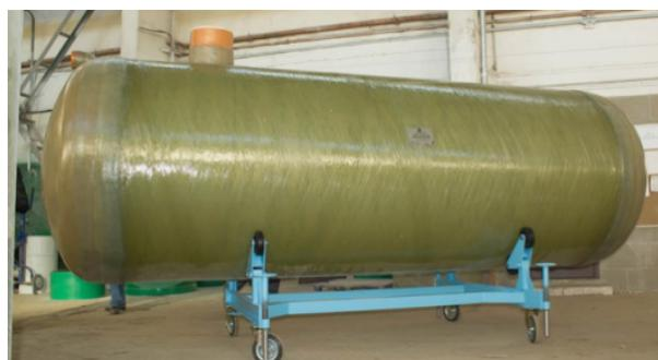
*Figure 2 – Fiberglass tank boiler obtained by winding*
