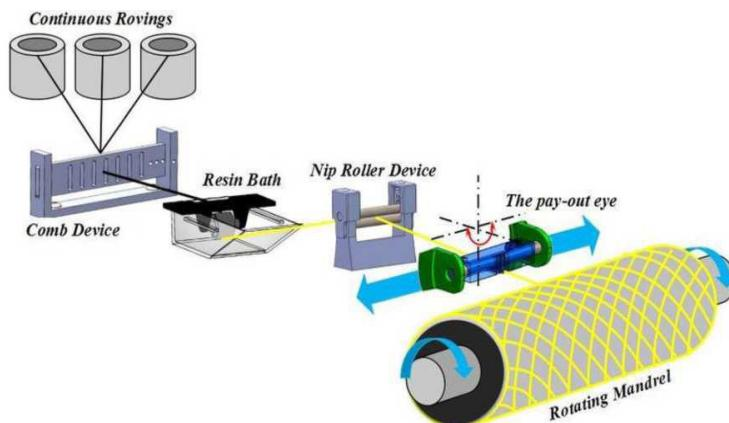
*Figure 1 – Process of winding the filament*
