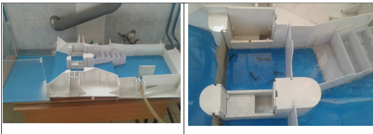
Figure 5 - Laboratory model of a fish pass 1:100.
