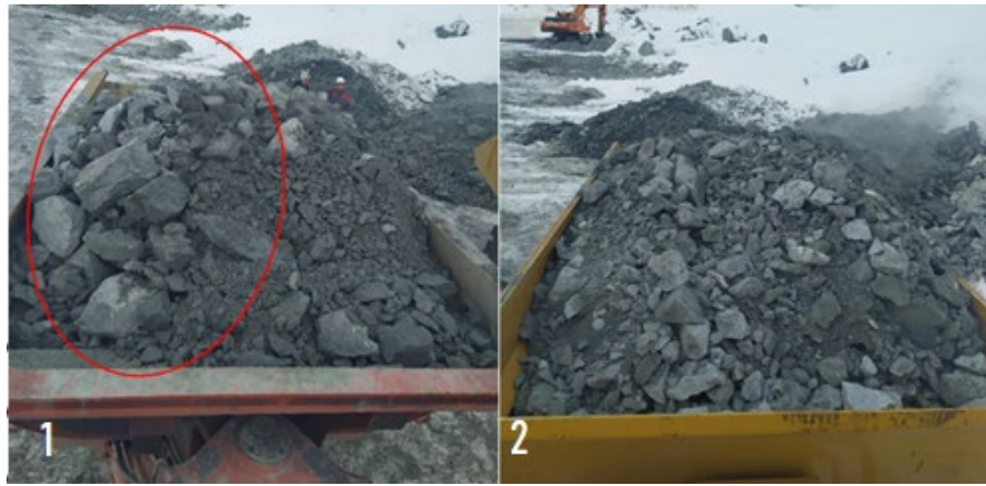
Figure 3. Photos of mountain masses in the bodies of loaded dump trucks on the surface. 1 – with the standard method, 2 – with the SPS method.
