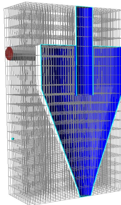
*Figure 3* - Calculation mesh of finite elements
