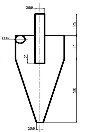
Figure 1 - Geometric characteristics of the hydrocyclone installation
