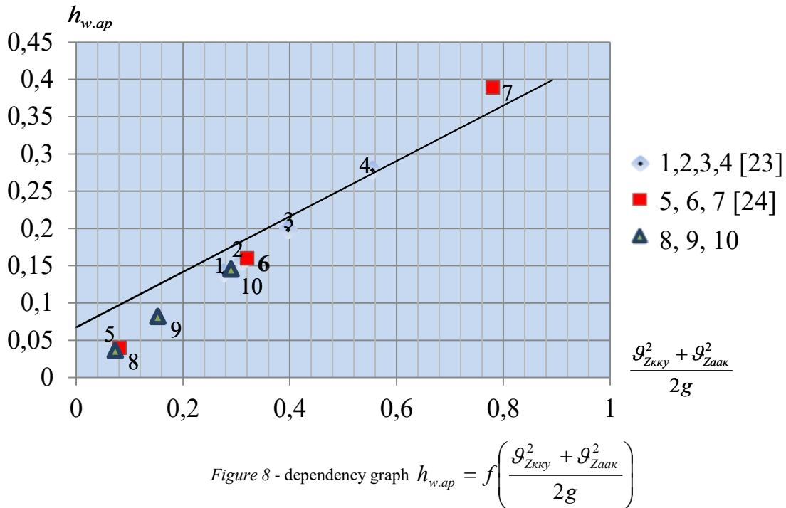
As you can see (Fig. 8)  $h_{w.ap}$  the pressure loss for mixing the flow in the conical part of the hydrocyclone
