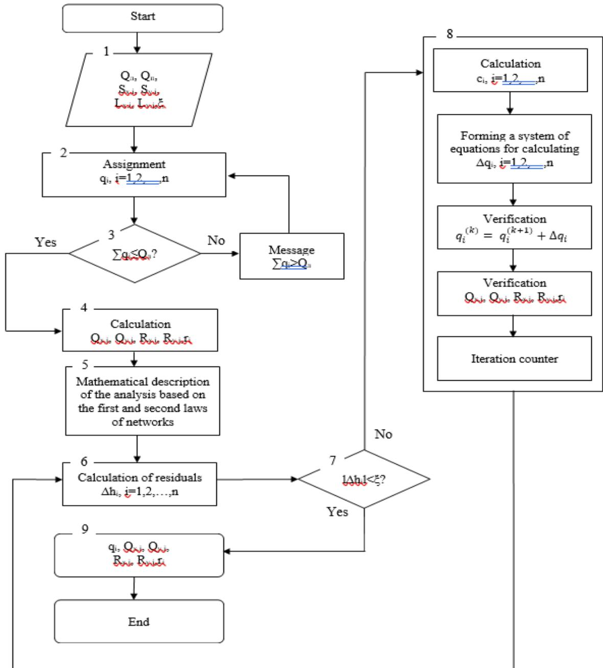
Figure 3 – Procedure of determining air losses
