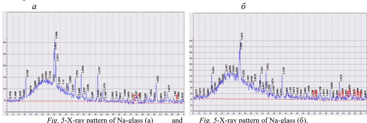
Fig. 5-X-ray pattern of Na-glass (a)
