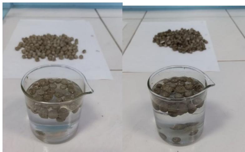
Fig. 4 - Granules of agloporite from Na-glass (Fig. 4, a) and from Na-Ca-glass (Fig. 4, b) float on the surface of water.
