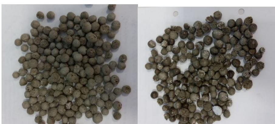
Fig. 2- Granules of Na-glass agloporite.      Fig. 3- Granules of agloporite from Na-Ca-glass.
