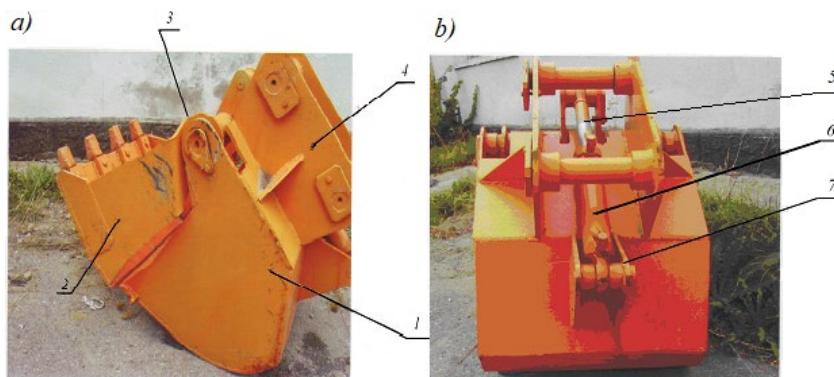
Figure 4. Excavator bucket design for development of coarse clastic soils of mudflows: a) - is a side view; b) rear view, 1- main bucket; 2 shows the opening part of the bucket; 3 - hinge; 4 - bracket for attachment of hydraulic cylinder; 5 - hydraulic cylinder rod; 6 - hydraulic cylinder; 7 - bracket
