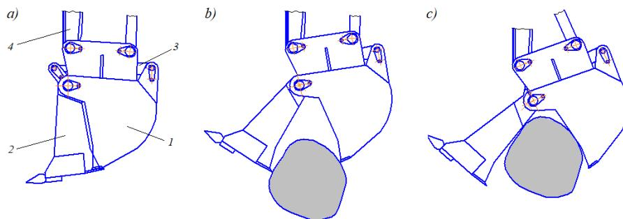
Figure 1. Technological operations of a single-bucket excavator equipped with a hydraulically controlled jaw for development of coarse elasic soils of mudflows: a) - is a general view of an opening jaw bucket; b)- filling process; c) - unloading process, 1-bucket; 2- jaw; 3- hydraulic cylinder; 4- handle
