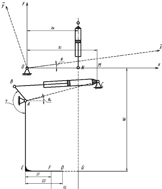
Figure 2. Kinematic diagram of bucket with jaw for development of coarse elasic soils of mudflows
