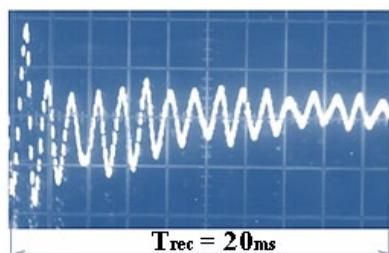
Figure 6 - The response of the system without correction for mechanical impact disturbance
