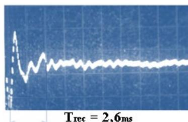
Figure 8 – The system response with the correction of its dynamic properties to mechanical shock disturbance
