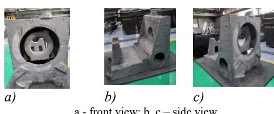
Figure 2 - Submersible pump frame
