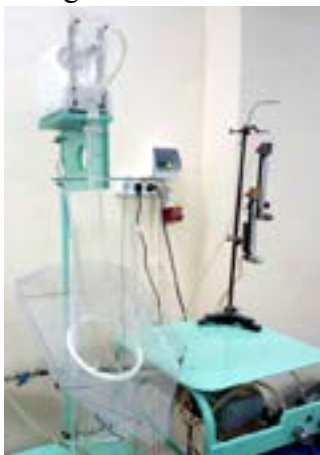
Fig. 6. – The laboratory installation of the column flotator with the pneumatic aeration of the liquid
