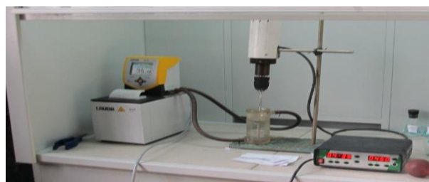
Figure 1: Working installation for the study of leaching on a mixer
